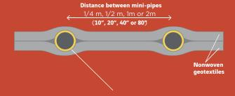
Perforated mini-pipes liameter 16 mm, 20 mm or 25 mm
