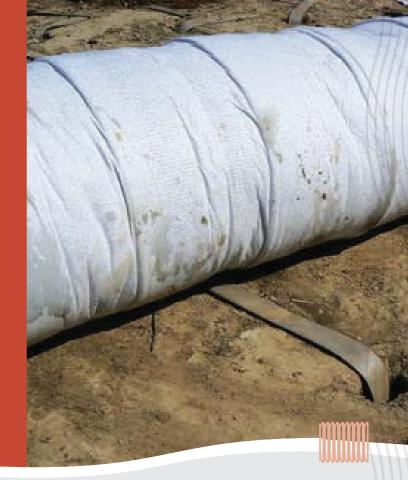
**DRAINTUBE™** is a combination of proven materials like various geotextile layers (filtration, separation and protection layers) and perforated mini-pipes that are needle punched together for high capacity drainage. It is manufactured as per the standard to ensure optimum performance under the most difficult conditions. Each roll performs the functions of separation, filtration and drainage essential for building better roads.
